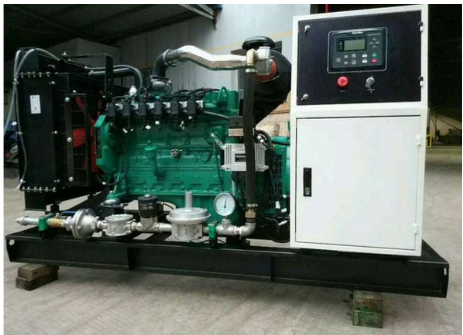
CNG Modeled Gas Generator
